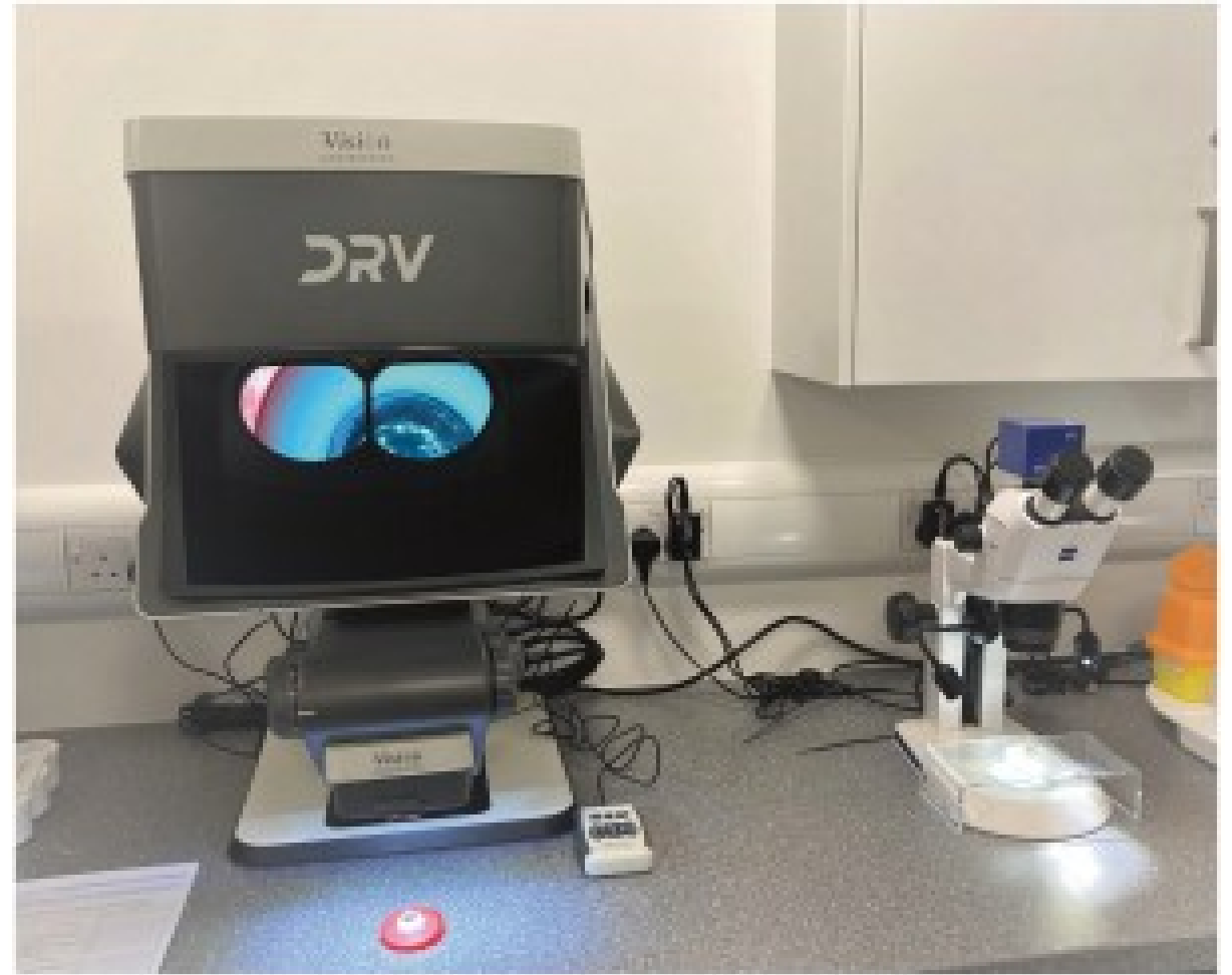
Fig. 1 Photo illustrating viewing equipment currently used for ophthalmic simulation in Glasgow. Note the larger image and heads up display of the DRV system compared to the smaller STEMI microscope.
